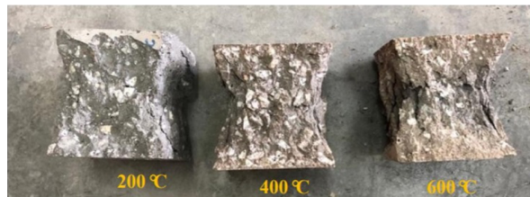
Fig. 7. Residual concrete cube sample with 25% RSA replacement after exposed to elevated temperature
